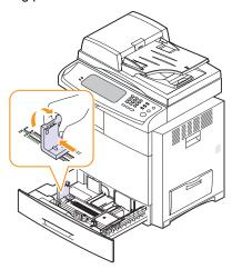
2 After inserting paper into the tray, while pinching the paper width guide as shown, move it toward the stack of paper until it lightly touches the side of the stack. Do not press the guide too tightly to the edge of the paper; the guide may bend the paper.
